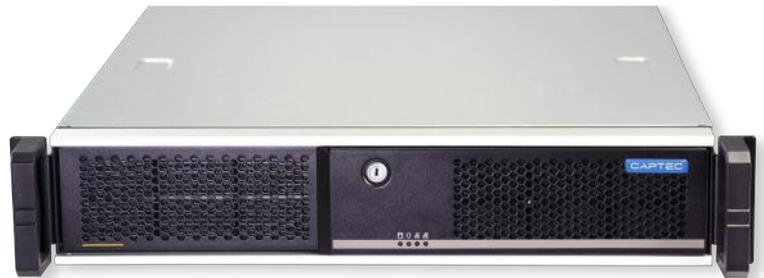
The new IC-425-S series from Captec is our most versatile off-the-shelf 2U platform. It combines the largest storage capacity of the IC range with a full complement of chassis security features and easily serviceable dust particle fan filters.
