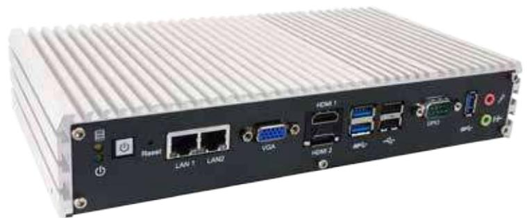
Reliable, powerful fanless rail computer with multiple I/O capabilities. Rugged construction with wide temperature range, shock & vibration resistance and small size provides a powerful computer for many rail vehicle and trackside applications.
