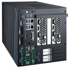
These highly expandable dual GPU workstations allow integrators to combine machine vision applications with AI. Powered by 6 core 8th generation Intel processors and leading edge RTX 2080 Nvidia Turing architecture, the workstation range delivers high processing performance for demanding real-time applications.
