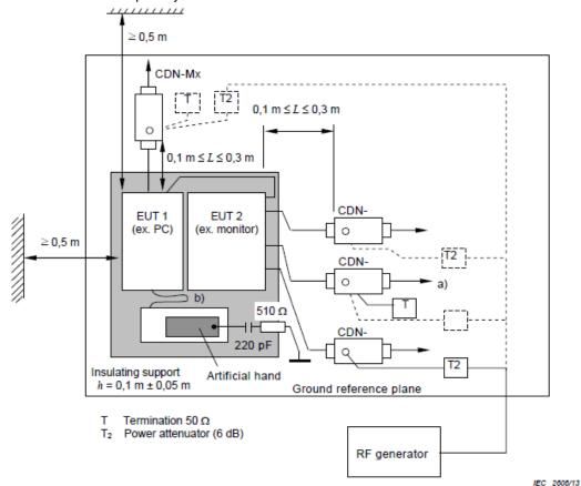
a) Only one of the CDNs not used for injection shall be terminated with 50 Ω, providing only one return path. All other CDNs shall be configured as decoupling networks.
